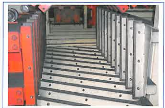
Anode long surface scraping
