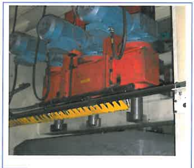
Anode stub hole cleaning
